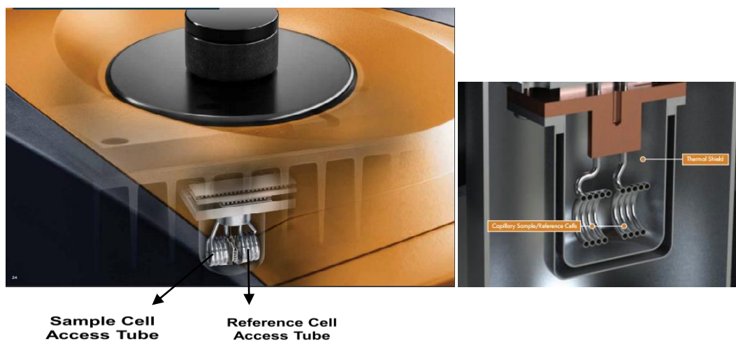
Figure 2: Representative diagram of a Differential Scanning Calorimeter experiment. The basic feature of Nano DSC instrument is reference and sample cell made to allow high temperature operation. Power is supplied to both the cell containing a resistance heater and temperature sensor to increase the temperature at constant rate. The difference between the power of the two holders is used to calculate DdH/dt
