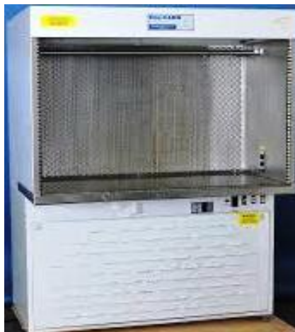
Fig. 3 An iodine fuming cabinet
