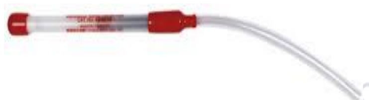
Fig. 2 An iodine fuming gun
