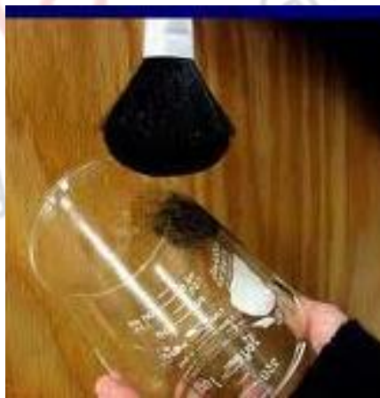
Fig. 4 Developing latent fingerprints by iodine powder
