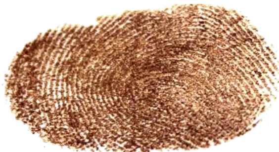
Fig. 1 A sample fingerprint developed by iodine fuming method
