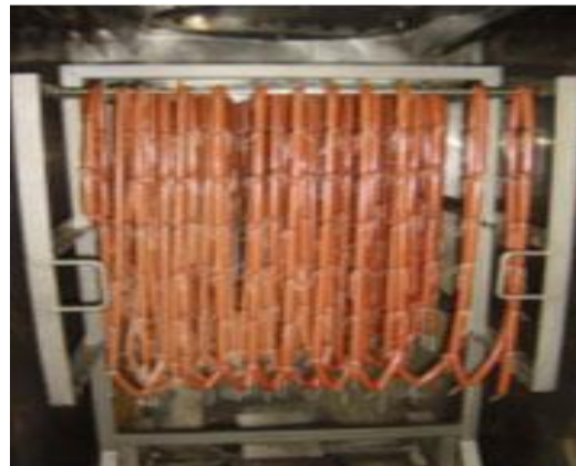
Fig.10: Hotdogs are placed in the smokehouse for hot smoking (pale colour before smoking) Fig.11: After completion of the smoking process (brown-red colour after smoking)
