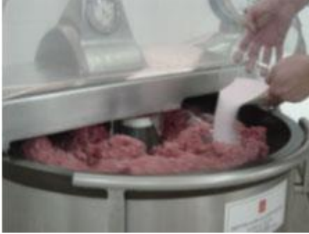
Fig.3: Adding of nitrite curing salt during initial phase of meat mix fabrication
