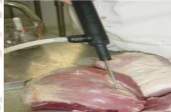
Fig.8: Brine injection with a manual curing pump
