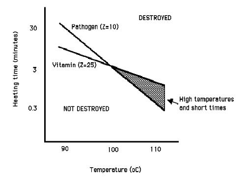
Alkaline phosphatase is a naturally-occurring enzyme in raw milk which has a similar Z value to heat-resistant pathogens. Since the direct estimation of pathogen numbers by microbial methods is expensive and time consuming, a simple test for phosphatase activity is routinely used. If activity is found, it is assumed that either the heat treatment was inadequate or that unpasteurized milk has contaminated the pasteurized product.
