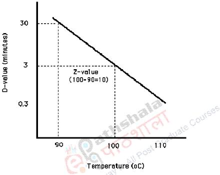
Reactions that have small Z values are highly temperature dependent, whereas those with large Z values require larger changes in temperature to reduce the time. A Z value of 10°C is typical for a spore forming bacterium. Heat induced chemical changes have much larger Z values that microorganisms, as shown below.
