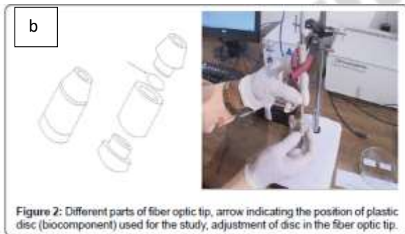
Figure 1: Optical biosensor for detection of Cd^{2+} ions (a) colour of sensing mixture before and after the urease activity, b) Assembly of biocomponent at the fibre optic tip.
