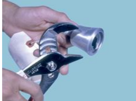
Fig2. Tool marks by an arc joint plier (Impressed tool marks)
