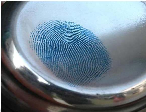
Fig. 2 A sample fingerprint developed by nanoparticle-size composition based on crystal violet stain on a steel article
