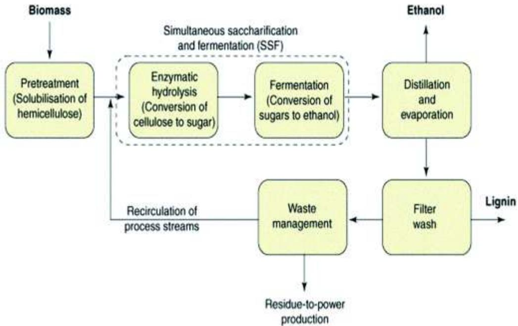
**Figure 1: Process flow of biomass to ethanol generation** (Source: [http://pubs.rsc.org/services/images/RSCpubs.ePlatform.Service.FreeContent.ImageService.svc/ImageService/Articleimage/2015/RA/c5ra12735a/c5ra12735a-f5\\_hi-res.gif](http://pubs.rsc.org/services/images/RSCpubs.ePlatform.Service.FreeContent.ImageService.svc/ImageService/Articleimage/2015/RA/c5ra12735a/c5ra12735a-f5_hi-res.gif))
