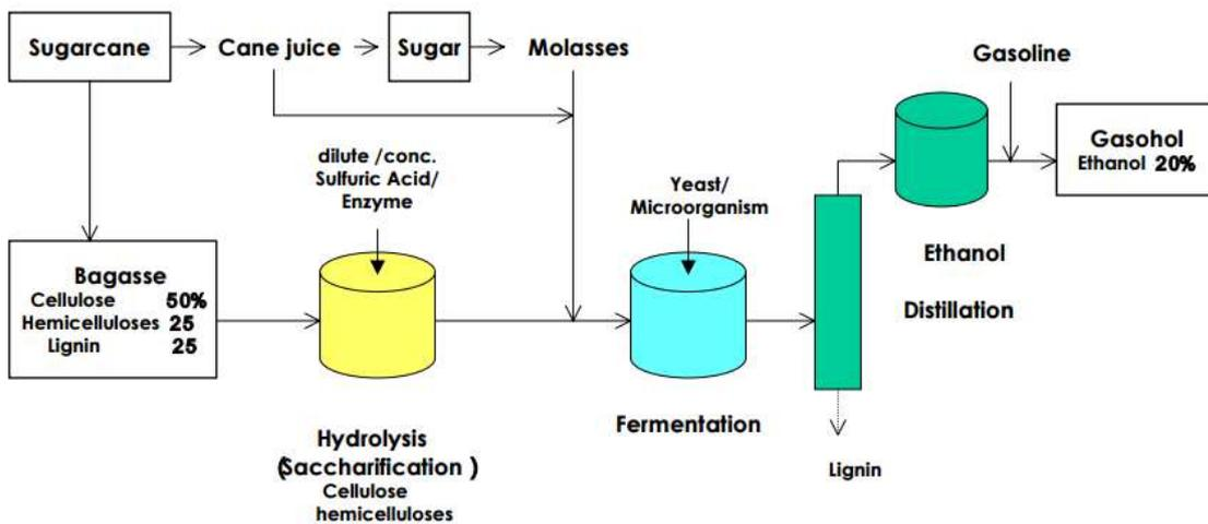
**Figure2 : Flow diagram of the ethanol production process** (Source: <http://www.ee-design.net/imgEED/IMG CUT/topics/topics20061214/sugarcane.gif>)
